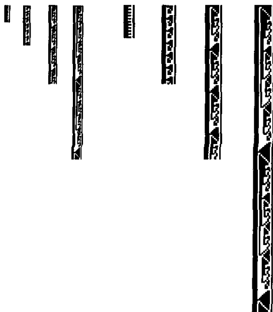
Figure 7. The first four periodic cylinders of example 2, with periods of 2, 8, 28 and 96. We see the operation of the barrier 01, which is always effective on the right and is effective of the left if the nearest 1 to the right of the D_0D is an even number of cells away.
